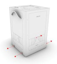
2. Unscrew all four locking screws of the wooden case cover while the speaker/case is in a vertical upright position.
