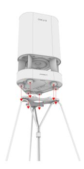
Make sure that the rubber feet of the speaker are aligned and inserted correctly into the designated stand top holes.
